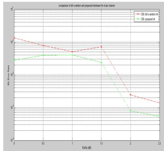
Figure 8. Comparison of BER Performances in Full S-random Interleaver and Proposed Interleaver for Rician Channel
